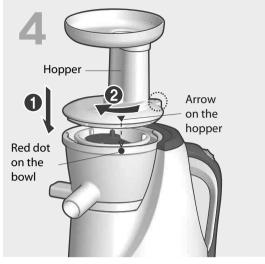
Assemble the hopper onto the bowl.
