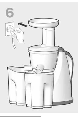
Now connect the power cord. Place a container under the pulp ejection and one under the juice ejection.
