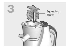
Place the squeezing screw in the center of the bowl and push tight.
