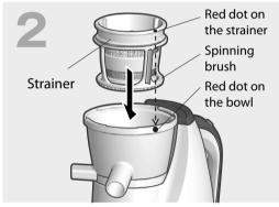
Assemble the strainer + spinning brush into the bowl.
