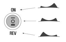
Turn off the machine and put in reverse for a few seconds. Then try operating again.
